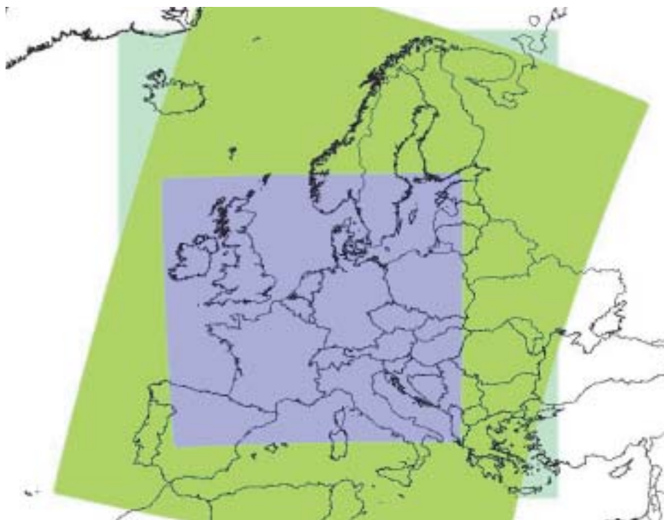
Figure 1 Spatial extent of the meteorological models used in the EFFS system. The DWD-LM model extent is shown in purple, the DMI-HIRLAM model extent in pale green and bounding box for the ECMWF-EPS archive retrieval in bright green.
